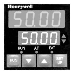
RUN - LED indicates that the programmer is in the run mode.
