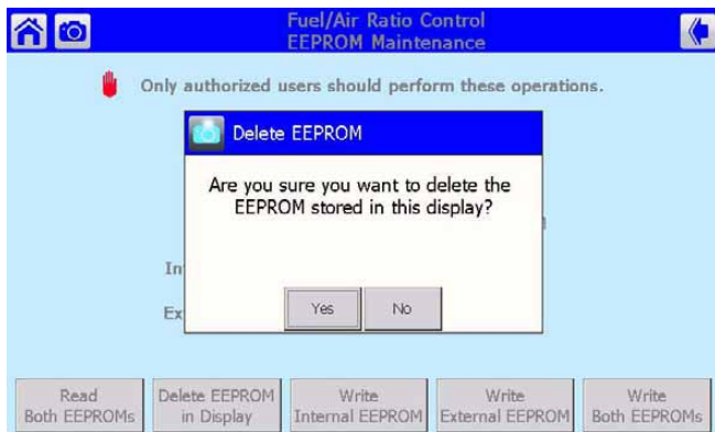
Fig. 74. EEPROM Maintenance—Delete Images from S7999D.
