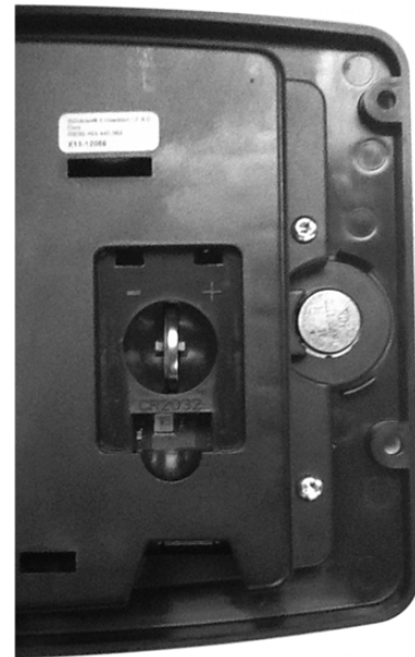
Fig. 15. Install CR2032 coin battery.
