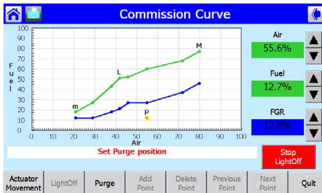
Fig. 57. Purge setting on Commission.
